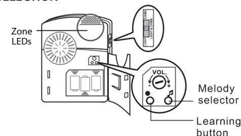
If the coding is successful, the chime will generate a short tone. If another LED lights up, this transmitter is already programmed on the zone that lights up.
