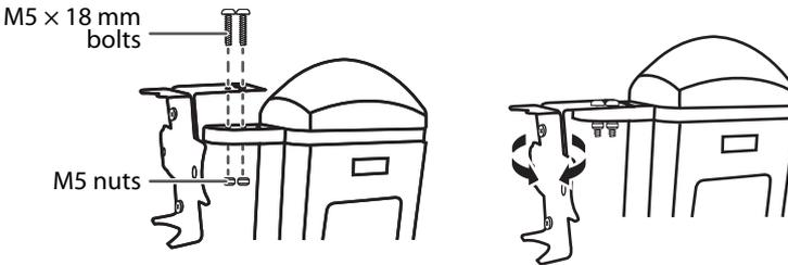
3. Mount sensor unit B first, attaching it to a post with two U-shaped brackets, four M5 nuts, and four M5 × 27 mm bolts. Tighten securely, making sure that the sensor is level and the IR windows are facing toward where you will mount sensor unit A.
