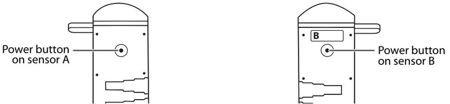
3. Test the transmitter by completely blocking all three IR windows. You should hear a click and the indicator light in the center window of sensor A lights.
